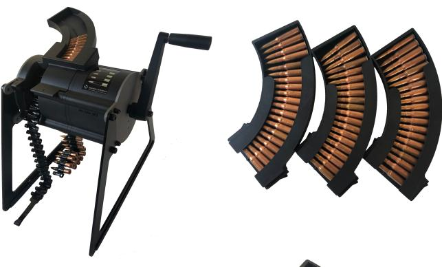
Link machine with a single row hopper for 20 rds allows you to link various types of ammunition in a specific order.
